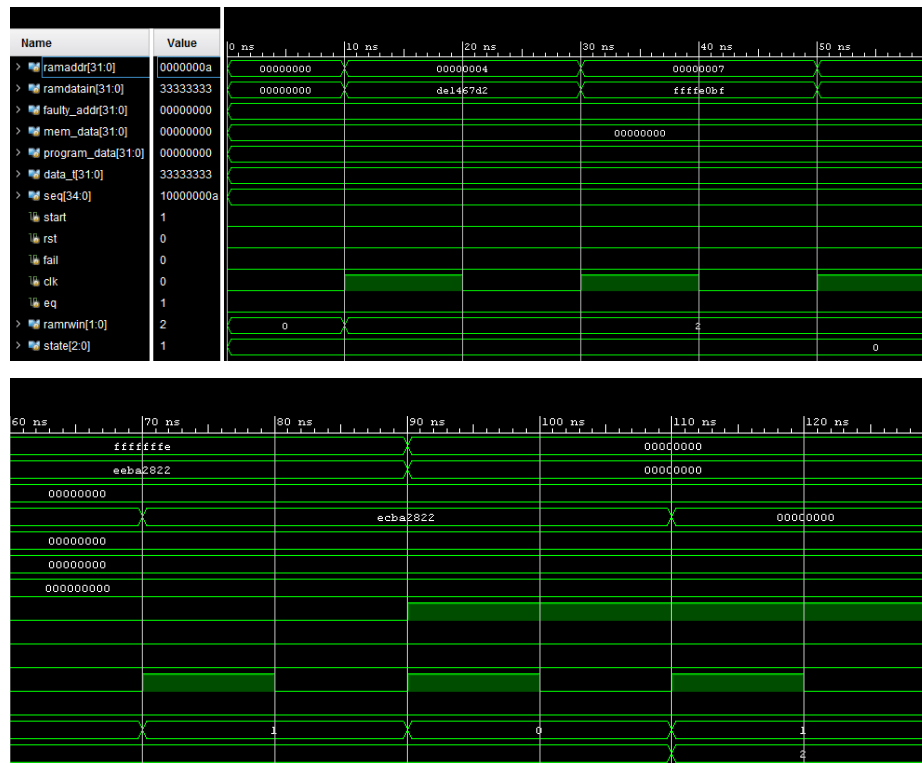
Fig 12A&B. Start of the MBIST Simulation. Runtime of Figure(s) is 0 to 120 ns
