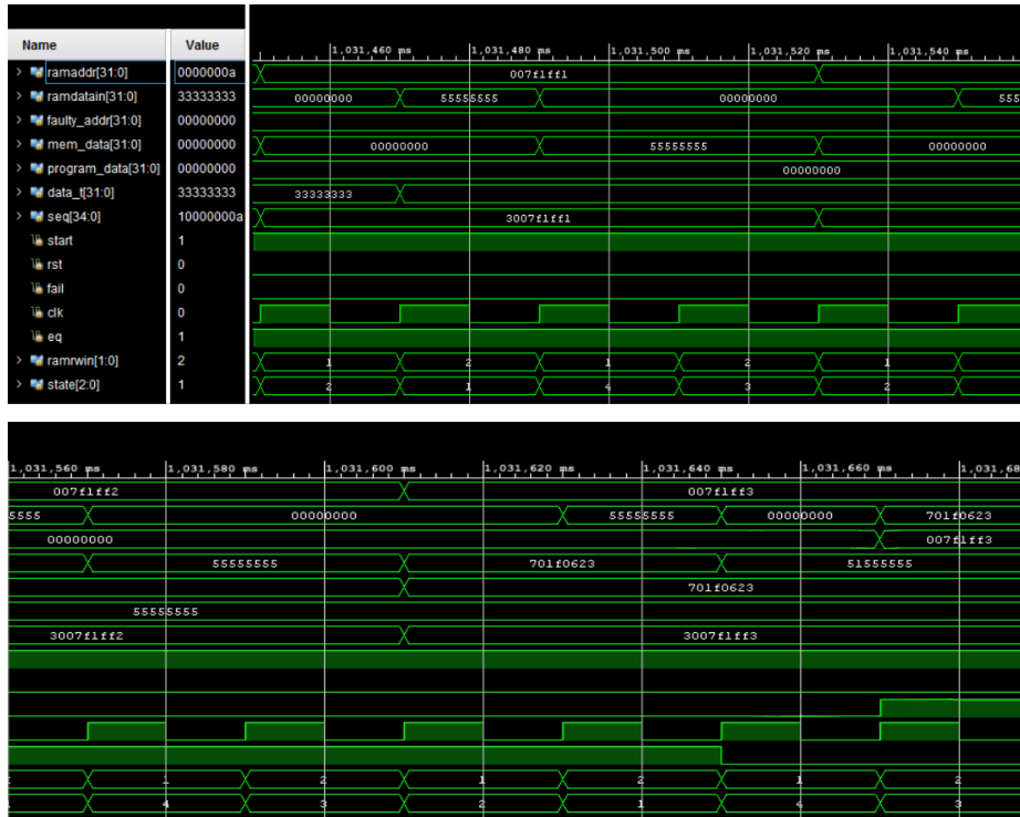
Fig 15A&B. MBIST Finally Catches Faulty Address and Sets Fail Flag High. Runtime of Figure is 1,031,455 to 1,031,680 ms.
