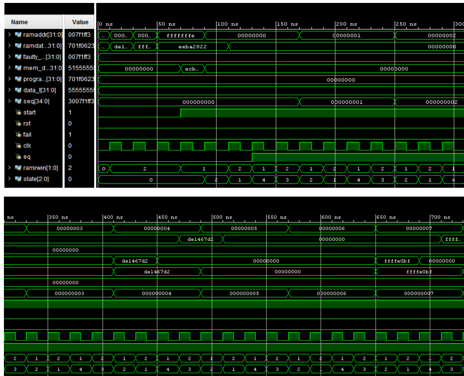
Fig 13A&B. Start of the MBIST Simulation and First 7 Addresses to be Tested. Runtime of Figure is 0 to 740 ns.
